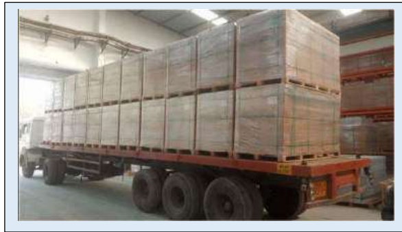
Fig.1 Before unloading, check all Pallets and Packing are good condition with no physical damage
