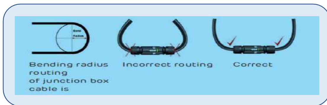
Fig.8.1 Recommended cable routing
