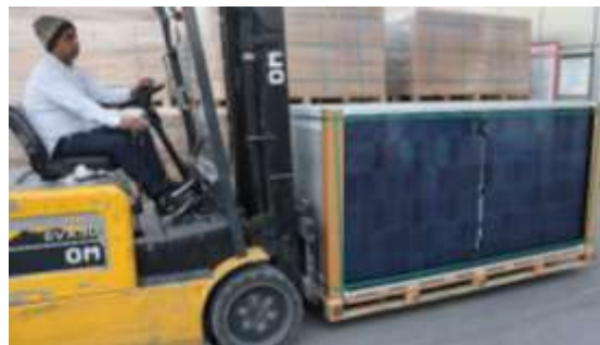
Fig.2b Please drive slowly and avoid allowing the forks to strike the cartons or pallets
